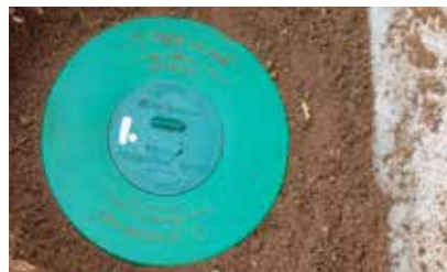
Photo 3. Sentricon RTI station correctly installed; sitting flush with the soil surface and with clearly identified station number.
